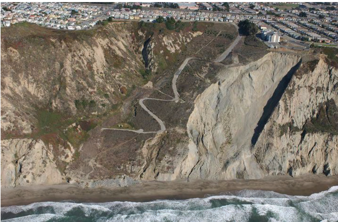
Figure 10. Aerial photograph of the landslide taken on October 5, 2005, after completion of the NBL investigation. Portions of the church property at the head of the landslide and blocks along the north margin have failed since landslide mapping was completed during 2004 (Figure 5). Note that a hairpin turn in the access road for the Avalon Canyon storm drain project was relocated in 2005, because slow, steady movement of headscarp blocks began to open releasing fractures and undermine a portion of the road. Published by permission of Kenneth and Gabrielle Adelman, California Coastal Records Project.
