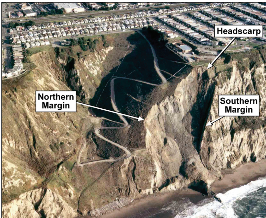
Figure 1. Oblique aerial photograph of the Northridge Bluff Landslide taken within two weeks after the December 2003 failure.
