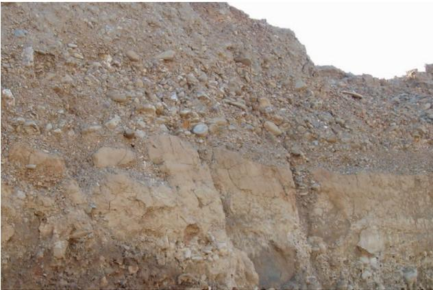
Figure 4. Sandy gravel over a fine-grained bed exposed in the shallow portion of the quarry pit wall.
