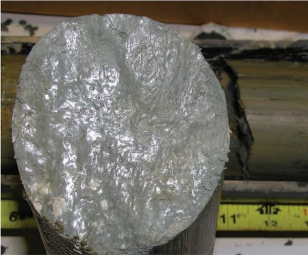
Figure 6. A core sample exposing a polished surface within the sheared unoxidized clay.
