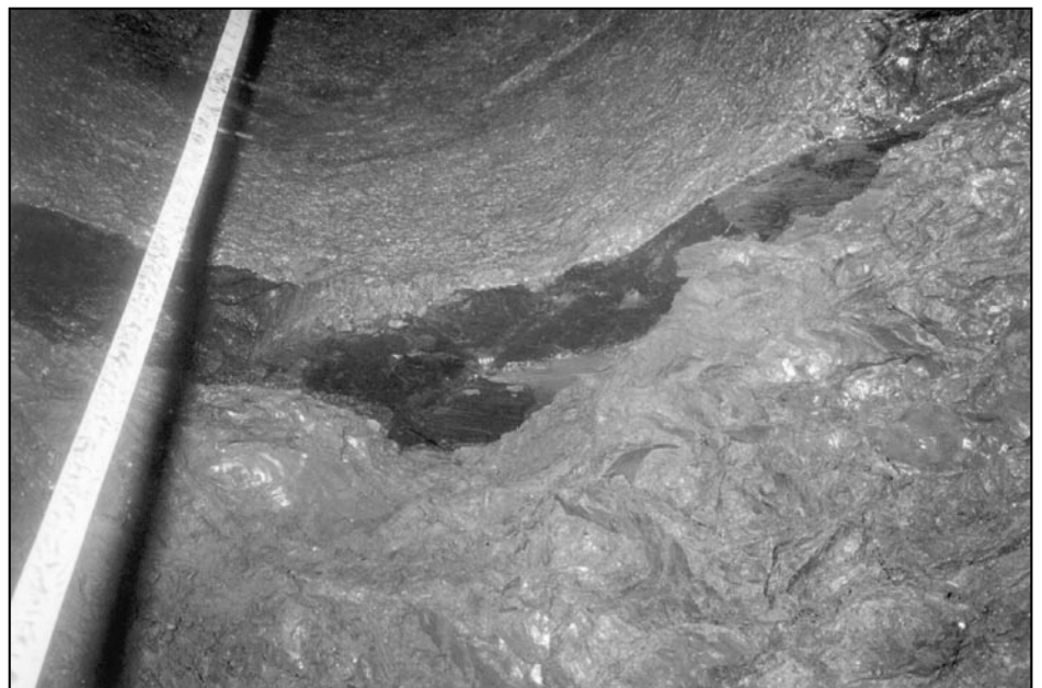
Figure 2. Photograph looking upward at gouge materials exposed below a polished bounding surface within a large-diameter borehole.
