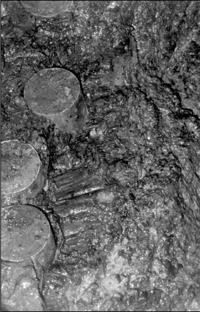
Figure 5. A photograph of shear zone samples. In this case, brass sample liners were driven into gouge materials that overlie a striated bounding surface.
